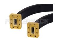
WR-90 Flexible Straight Waveguide Section 12 Inch Length with CPR-90G Flange Operating from 8.2 GHz to 12.4 GHz
