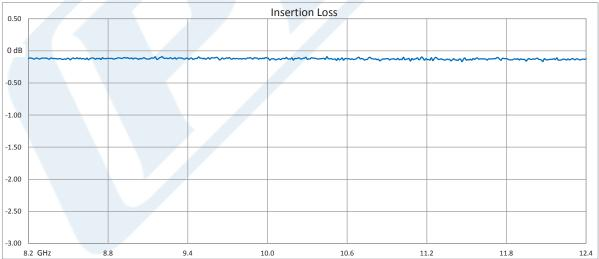
Click the following link (or enter part number in "SEARCH" on website) to obtain additional part information including price, inventory and certifications: WR-90 Flexible Straight Waveguide Section 12 Inch Length with CPR-90G Flange Operating from 8.2 GHz to 12.4 GHz PE-W90SF006-12
