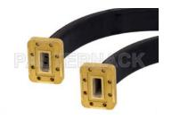
WR-90 Flexible Straight Waveguide Section 12 Inch Length with CPR-90G Flange Operating from 8.2 GHz to 12.4 GHz
